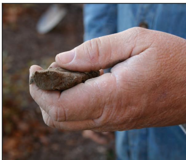
Figure 43. Roll the ball between your hands to make a rope of soil uniformly thick. If your rope breaks before extending an inch then you probably have sandy soils that allow proper drainage. This site may be suitable for your rain garden.
