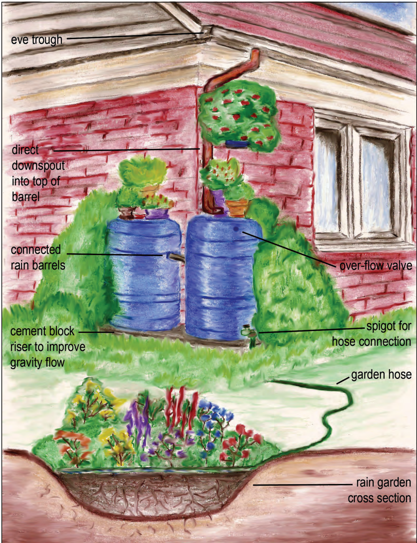
Figure 33. The drawing above illustrates how rain gardens and rain barrels work together to capture runoff. The downspout is directed into a rain barrel to collect roof runoff. In order to collect more roof runoff, two rain barrels are connected to each other. The excess runoff will pour out through the rain barrel's over-flow valve. You can attach an overflow hose to the valve to help direct flow towards your rain garden. By storing the stormwater runoff in rain barrels, you'll be able to water your rain garden during dry periods.
